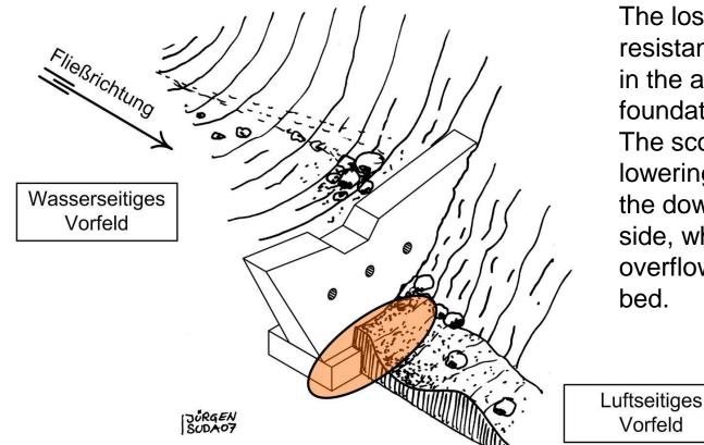
The loss of lower resistance occurs in the air-side foundation area. The scour or a bed lowering forms on the downstream side, where the overflow jet hits the bed.
