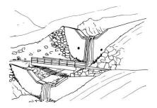
1. Building types of protective structures for torrent control
